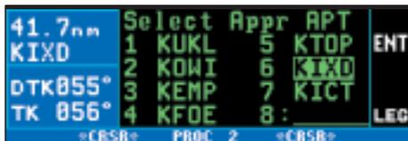
2. When "Approach" is chosen from the menu, the KLN 94 displays a list of airports in the active flight plan, along with other airports having approaches that are close to the aircraft's current position.
