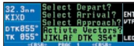
5. When the controller begins providing vectors, press the "PROC" button to display the FAF (JIKLA) and its course (354°). Press the "ENT" button, and the KLN 94 activates vectors and makes JIKLA the active waypoint and 354° (the course to it.) That's all there is to it!
