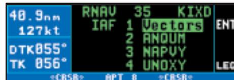
4. When radar vectors are to be provided by ATC, choose "Vectors" in place of a published initial approach fix to intercept the inbound course to the final approach fix. This loads approach waypoints into the active flight plan, beginning with the final approach fix (FAF).
