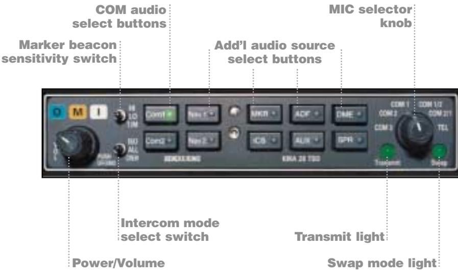
Then, there are such intercom features as IntelliVox®\* automatic squelch control, with separate voice activated squelch circuits for each microphone input to eliminate intercom squelch adjusting; the convenience of 6 intercom stations; and the real pleasure of stereo entertainment outputs.
