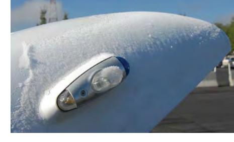
quantities—plays havoc with that balance. Ice reduces lift while it increases both weight and drag. In a typical light general aviation airplane, you are very unlikely to have sufficient thrust to overcome those penalties.
